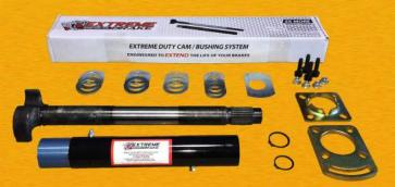
Includes Extreme Brake S-Cam & Universal Mounting Hardware (fits most axles) \*Comparison based on 24" x 1.5" S-Cam. Actual bearing surface will vary by length.
